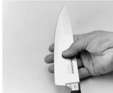
Figure 7. Burr can be detected by sliding fingers across and away from the edge.
